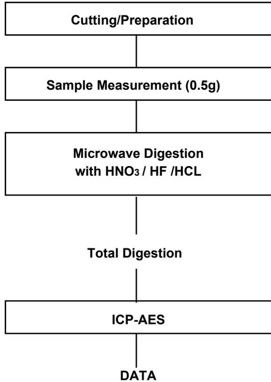
The samples were dissolved totally by pre-conditioning method according to above flow chart.
