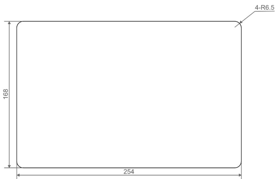
2. Drill a hole on the cabinet according to the hole size of step1.
