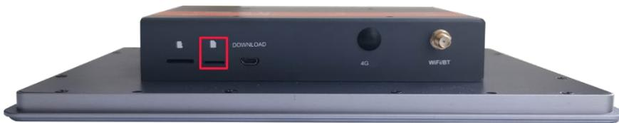
2. Insert the Nano SIM card into the corresponding card slot with the chip side up, and hear a sound to indicate that the installation is complete.
