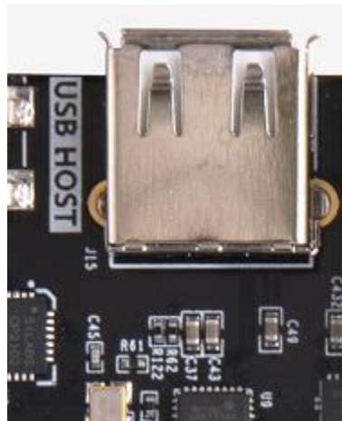
Figure 3-5-2: USB2.0 on the carrier board
