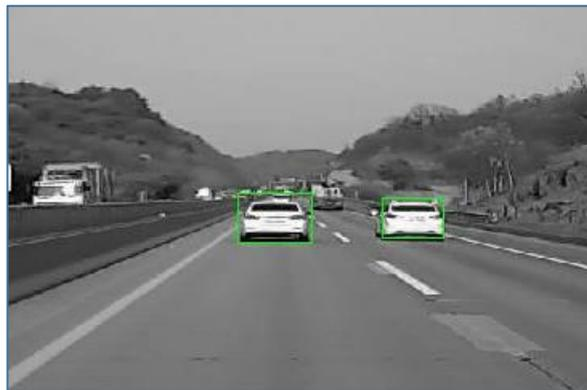
Compute Time-To-Collision (TTC) to warn or alert car collision
