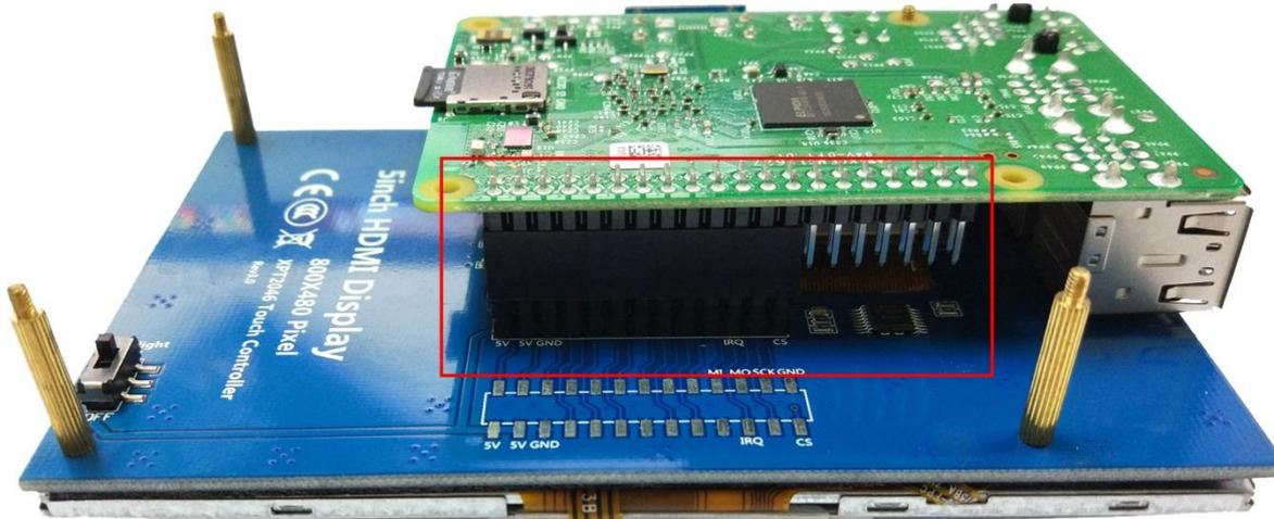
1) Connect The LCD 13\*2 Pin socket to Raspberry Pi as the Picture show above.
