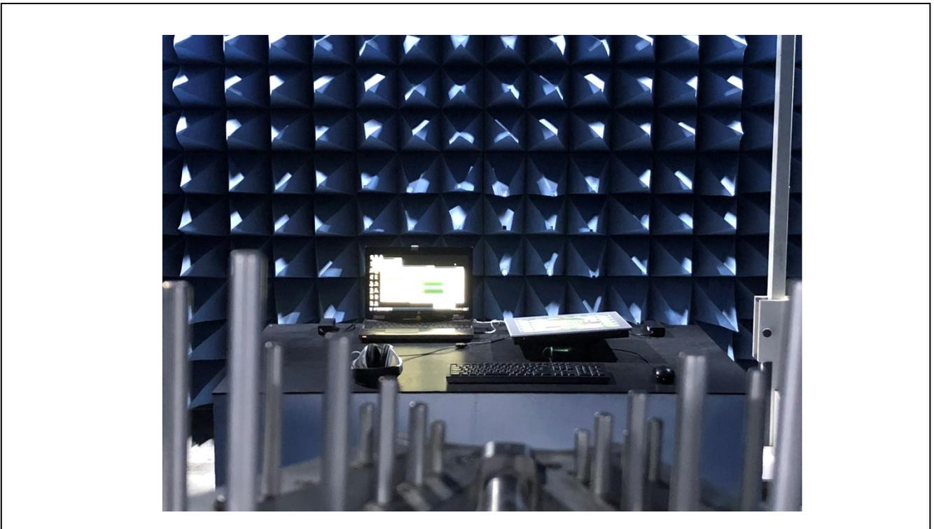
**APPENDIX IX - TEST SET-UP PHOTO: Electrical fast transient/burst immunity**
