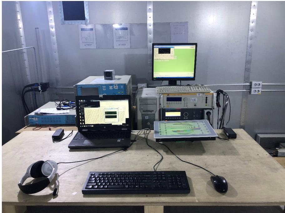
**APPENDIX XI - TEST SET-UP PHOTO: Conducted disturbance induced by RF fields Immunity**
