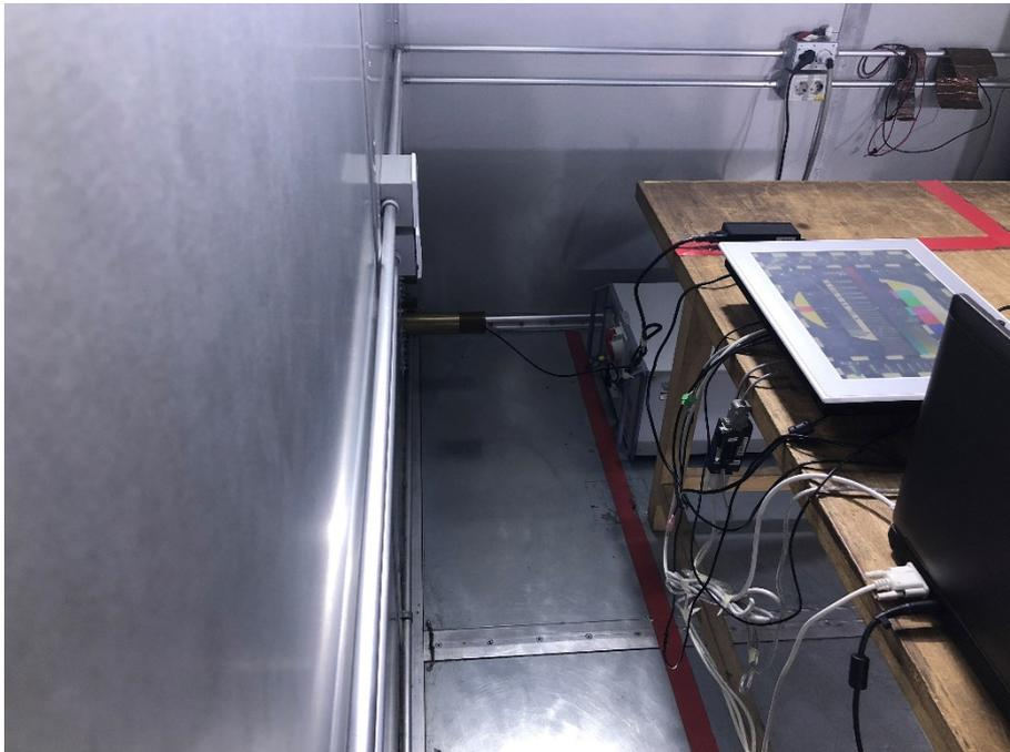
**APPENDIX II - TEST SET-UP PHOTOS: Conducted common mode disturbance at TEL ports**
