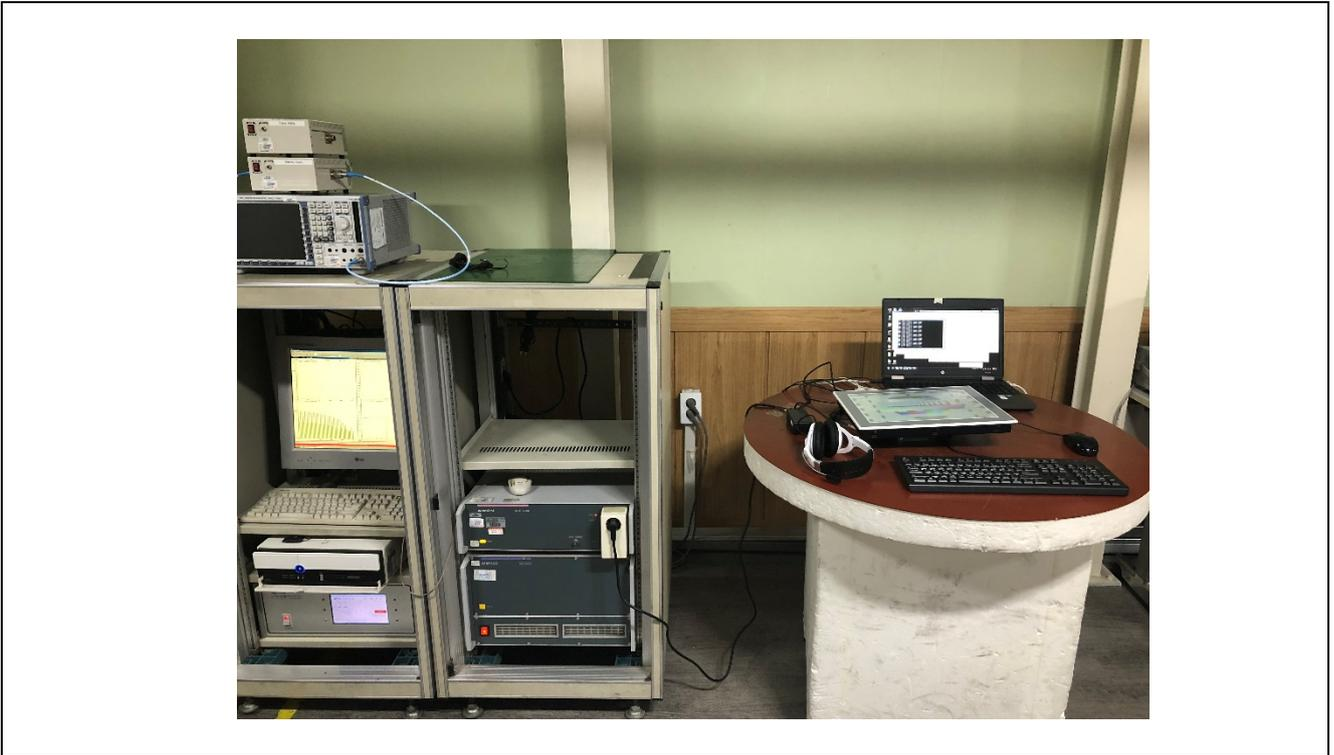
**APPENDIX VI - TEST SET-UP PHOTO: Voltage changes, Voltage fluctuations and Flicker**
