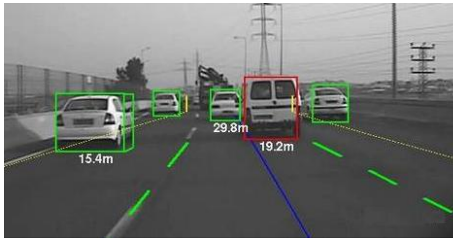
Figure 5 MR76 77GHz MMW Radar Application Illustration
