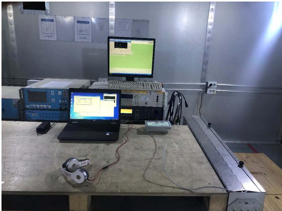
**APPENDIX VII - TEST SET-UP PHOTO: Conducted disturbance induced by RF fields immunity**
