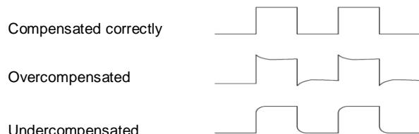
3. If necessary, use a nonmetallic screwdriver to adjust the variable capacity of your
