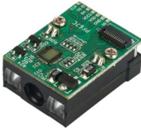
DE1400 is a practical embedded barcode scanner module with leading CCD image recognition technology and intelligent image recognition system. It can scan universal 1D codes, support USB, TTL, PS2 multiple interfaces, read the paper, goods, screens, other media barcodes. Easily embedded in a variety of OEM products handheld, portable, fixed and barcode collector, etc.
