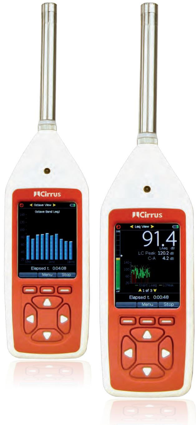
The  $L_{Ceq}-L_{Aeq}$  (C-A) value is also measured which can be used to select PPE using the HML method.
